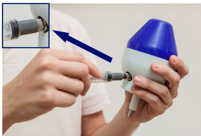
Figure 5-9: Connecting the Air Removal Tool
