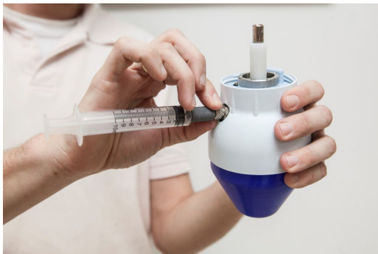
Figure 5-10: Opening the Water Port
