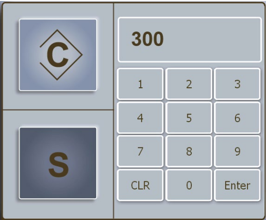
Figure 3-8: Window for presetting the Countdown
