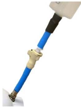
Figure 5-4: Attaching the syringe to the SWA
