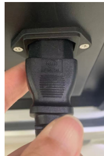
Power Supply Installation
